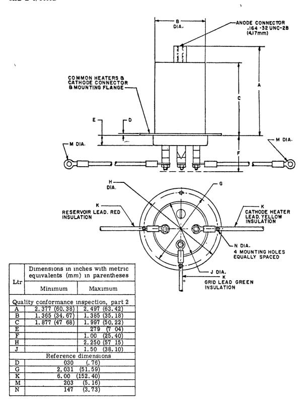
FIGURE 1A. Outline drawing of electron tube type 7665A.
