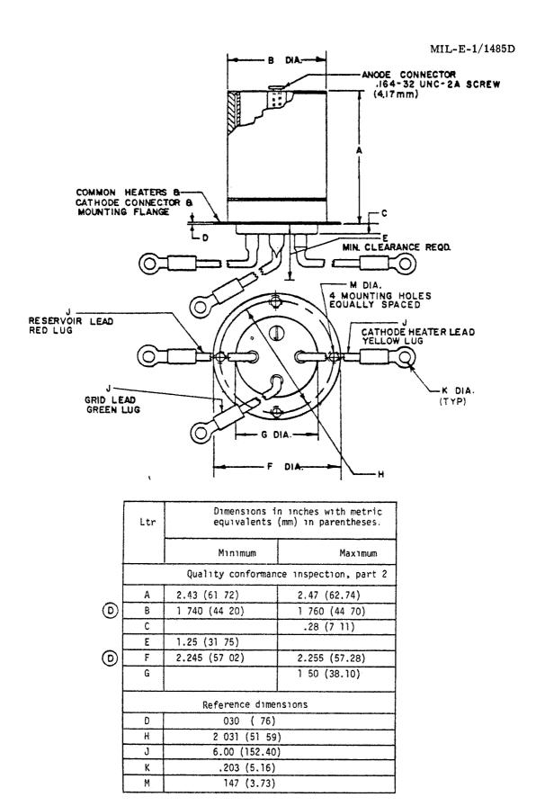
FIGURE 1. Outline drawing of electron tube type 7665.
