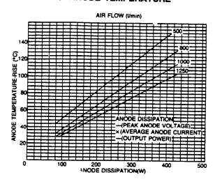
(Increase of anode temperature above inlet air temperature, T, as a function of anode dissipation, W, Anode dissipation = (peak anode voltage) × (average anode current)-(output power))
