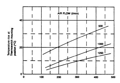
(Increase in temperature of thermoswitch mounting position above inlet air temperature, T, as a function of anode dissipation, W.)
